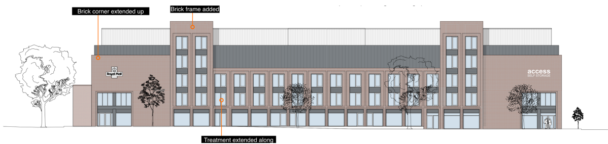
Detail of proposed new frontage of building
